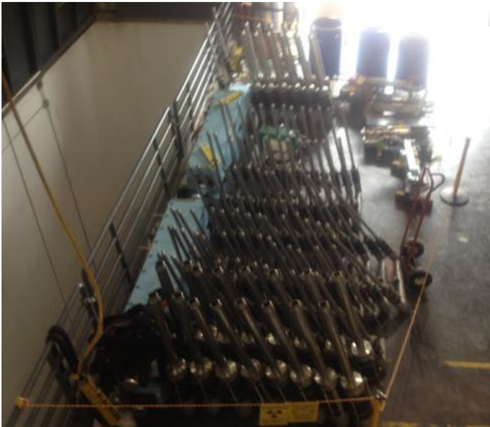
U-tubes awaiting rad survey
